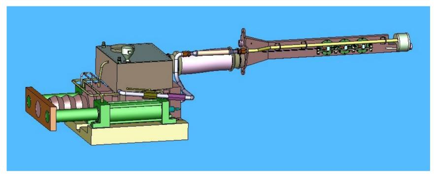
Double Containment System, with snout inserted into magnet.
