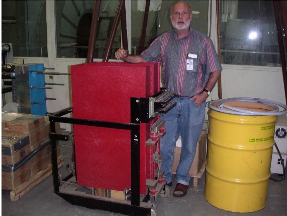
Mechanical Switch capable of 4.4 MW Pulsed System
