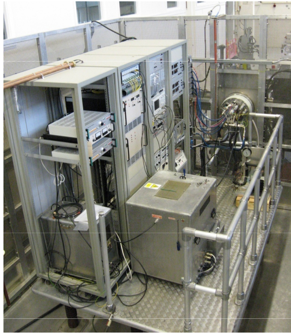
The FETS ion source installation
