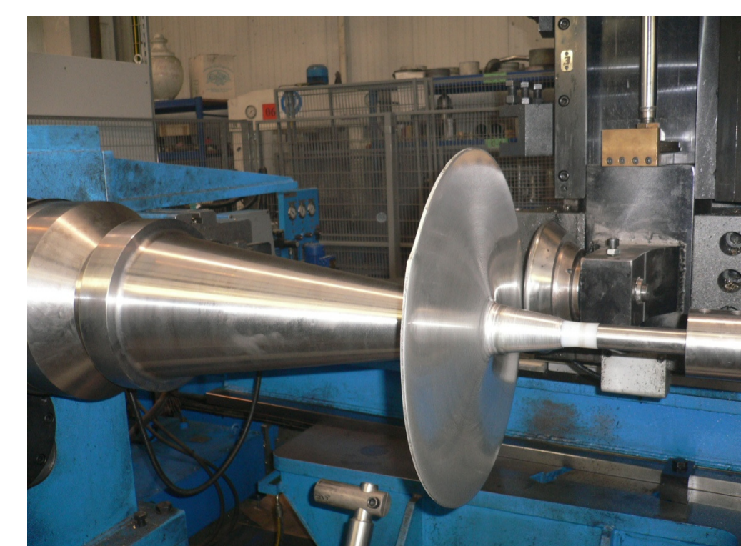
Design of the 18 kW beam dump (above) and spinning of the ultra-pure Aluminium (left)
