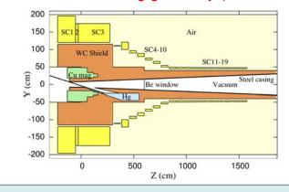
Superconducting coils (SC) in Study 2a geometry experience a radiation dose that is too high for their safe operation. Increased shielding in the new baseline geometry reduces the peak energy density in the SC coils to below 0.05 mW/g, equivalent to an integrated radiation dose of  $10^6$  Gy/yr, well below the maximum allowed dose of  $3 \times 10^7$  Gy/yr (operational lifetime  $\geq 10$  years) [3].
