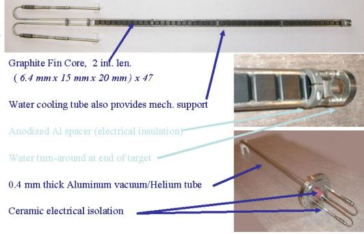
R&D in progress towards a 2-MW target.
