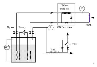
Figure 7: Scheme of cooling of the 15-T pulsed magnet via flow of He gas that is passed through a  $LN_2$  heat exchanger [8].
