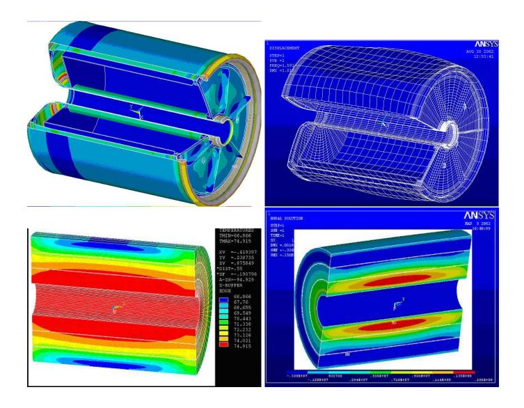
Figure 6: Top: structural analyses of the cryostat. Bottom: thermal and structural analyses of the coils. From [7].
