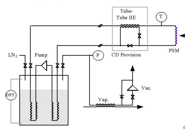
Figure 7: Scheme of cooling of the 15-T pulsed magnet via flow of He gas that is passed through a LN<sub>2</sub> heat exchanger [8].
