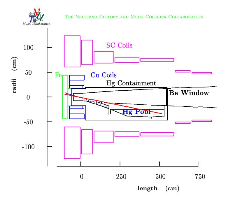
Figure 1: Concept of targetry based on a mercury jet and proton beam at 100 mrad and 66 mrad, respectively, to the axis of a 20-T solenoid magnet.
