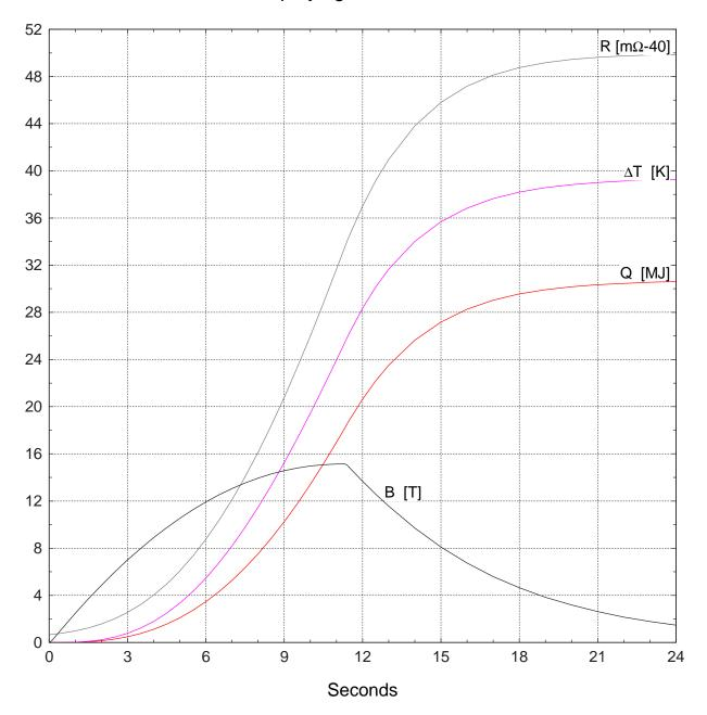
Figure 4: Behavior of the 15-T magnet during a pulse. The peak current is 7200 A at a peak voltage of 600 V. Approximately 30 MJ of energy is dissipated in the magnet, which raises its temperature from 70 to 110K.
