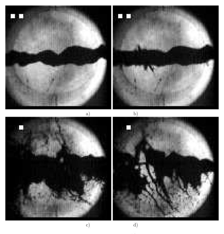
Figure 2: Hg jet interaction with  $3.8 \times 10^{12}$  24-GeV protons; t = a) 0 ms; b) 0.75 ms; c) 10 ms; d) 18 ms.
