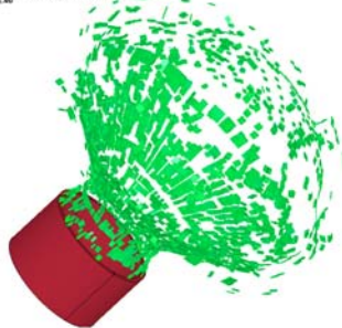
PMT Implosion Prediction - NUWC Test Time = 2.48
