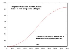
Figure 3. Temperature rise from a single pulse in a stainless steel window.
