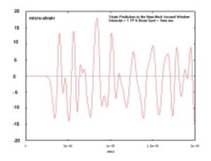
Figure 20: Predicted strains in the 6mm-thick Inconel 718 window
