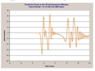
Figure 13: Predicted strains (ANSYS) in the 10 mil aluminum window for 2.5 TP and 1mm radius beam
