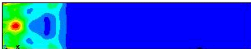
von Mises stress 1.2 micro-secs after pulse
