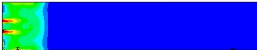
von Mises stress 700 nanosecs after pulse
