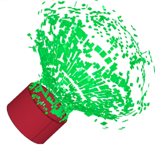
PMT Implosion Prediction - NUWC Test Time = 2.46
