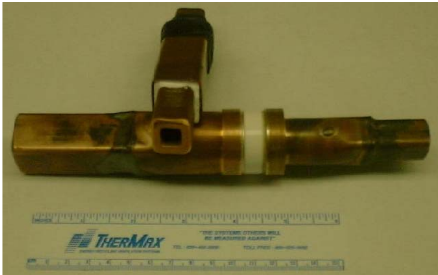
Fig. 9. Mineral-insulated hollow conductor developed for Japan Hadron Facility. 31 The end-on view shows the white layer of powdered MgO insulation sandwiched between the copper hollow conductor and its sheath, also of copper. The conductor is 18 mm square with a 10-mm square cooling hole. The MgO is 1.8-mm thick, and the outer copper sheath, 1.1 mm, for an overall dimension of 23.8 mm. Of the cross section, 17% is cooling passage, 37% conductor, 28% insulation and 18% sheath. The side view shows a conductor termination, brazed of several parts that confine the MgO and hold the glossy white ceramic ring that keeps the sheath isolated from the current-carrying conductor.
