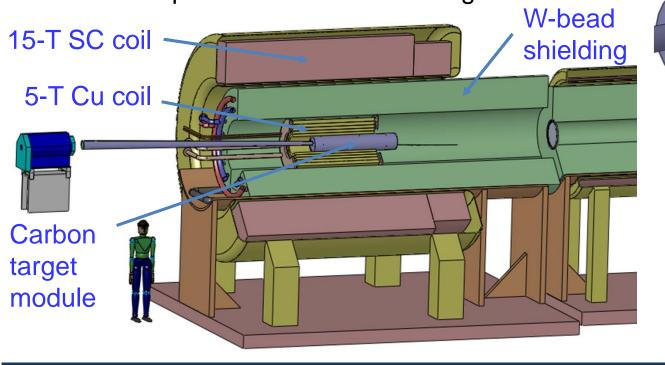
Next steps: simulate energy deposition to determine viable shielding scenario for the superconducting coils (including the chicane).
