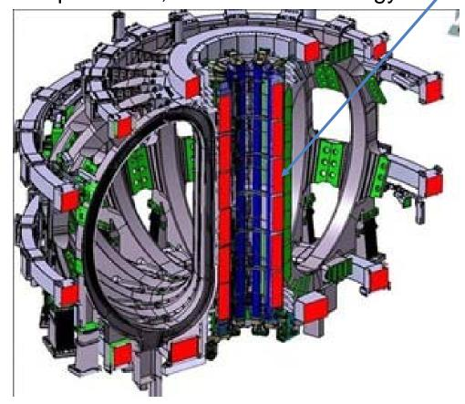
A high-temperature superconducting insert of 6+ T is appealing for our application - but its inner radius would also have to be large to permit shielding against radiation damage.
