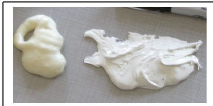
“Great Stuff” Home insulation foam survived the dunk tests very well. The white CTD material, applied in a thick coat, lost its bond after a dunk test, but behaved well as an adhesive. “Great Stuff” is flammable
