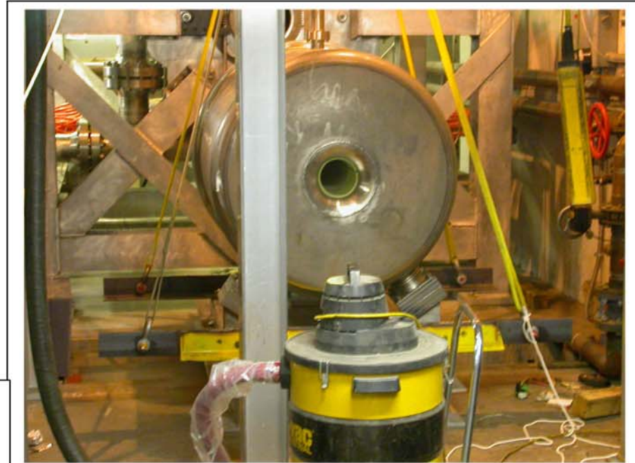
Magnet lowered into place in front of PTF split pair magnet.
