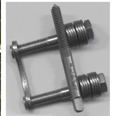
LN2 Dunk Test: Feb 9 2006 The gland for the power lead did not shatter – but it was rigid.
