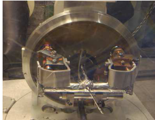
Figure 3.4: ... and after, where the cylindrical target (lower cylinder) is shifted by about 2 cm in forward direction of the beam.
