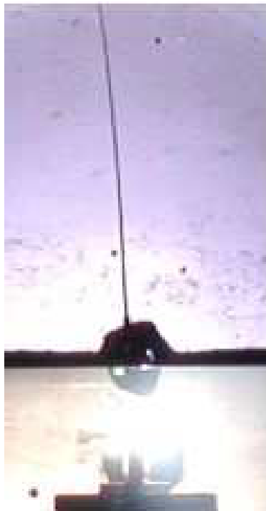
Figure C.1: Water vapor bubble collapsing close to the free surface. The velocity of the micro jet was not measured. A liquid dome is formed around the micro jet.
