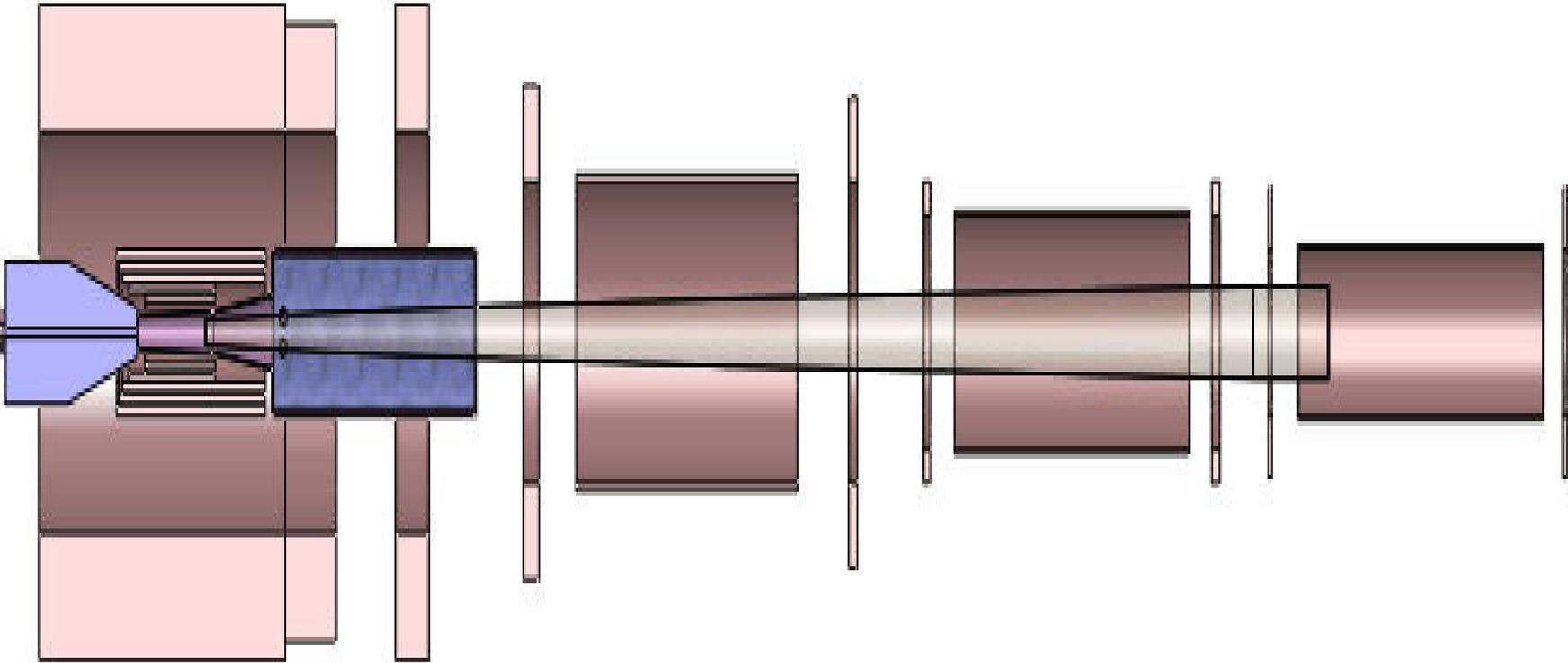
Target Magnet IDS120j: three solenoids per cryostat; large axial gaps at  $z = 4, 10, 15$  &  $20$  m [drawing courtesy Van Graves]. Target Magnet IDS120k is very similar, but the outboard solenoids in all cryostats except the first are of optimized (larger) inner radius, to improve field profile.  $U = 3.34$  GJ.
