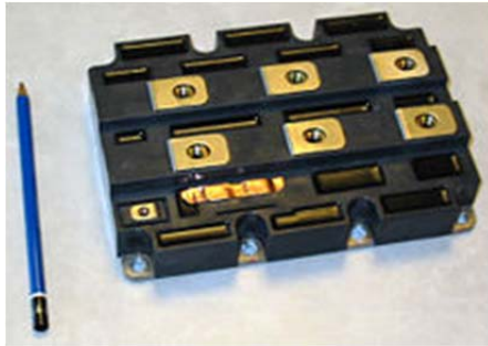
IGBT-Module (IGBTs and free wheeling diodes) with a rated current of 1,200 A and a maximum voltage of 3,300 V
