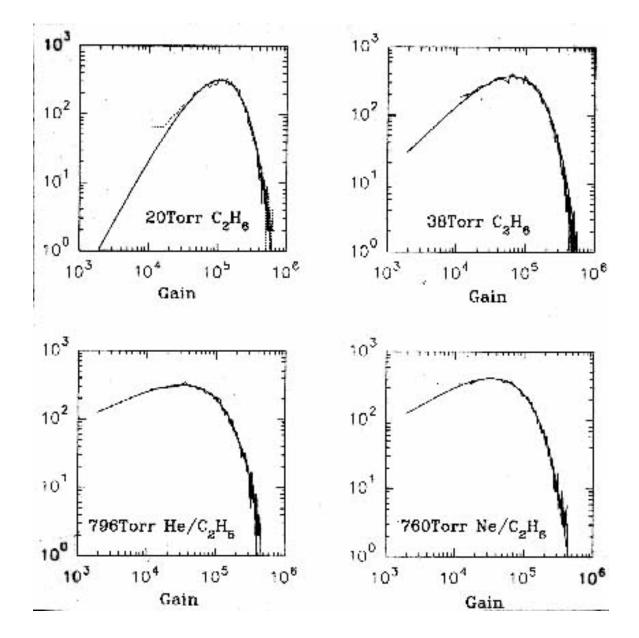
Can gain additional stability by adding helium as a buffer. [C. Lu *et al.*, NIM **A334**, 328 (1993).]
