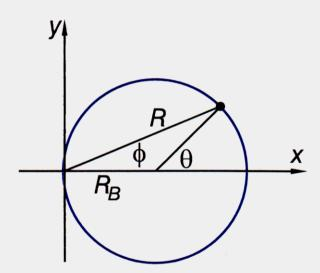
In a frame that rotates with angular velocity  $\omega_L = e\beta_z B_z/2P_z$ the orbit is a sine wave about the solenoid axis.
