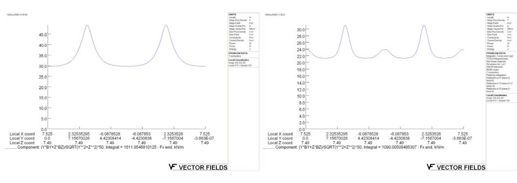
The largest force component => drives the mechanical design. ~60% lower force with iron.
