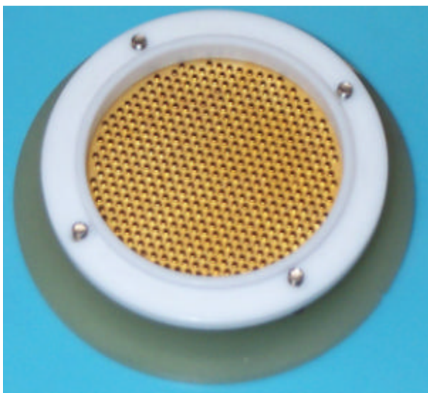
Figure 26 The CsI coating setup, which is placed in a vacuum deposition chamber for coating at CERN.
