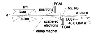
Figure 7. Layout of SLAC E-144 in which a tera Watt laser collides at  $17^\circ$  with a 46.6 GeV electron beam to produce backs cattered photons, electrons and positrons via nonlinear QED processes.
