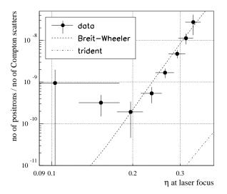
Figure 12. Rate of positron production in reaction (7), normalized to the total Compton scattering rate, as a function of laser field strength. Background from the trident process,  $e + n\omega_0 \rightarrow e'e^+e^-$ , is calculated to be negligible. About 2-3 ×10<sup>-10</sup> positrons per Compton scatter arise from interactions of backscattered laser photons with beam gas.
