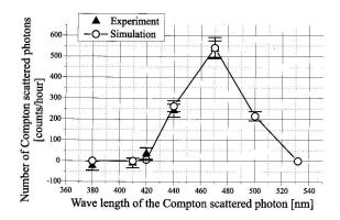
Figure 10. The wavelength of second harmonic scattering in the collision of an 800-nm Ti:sapphire laser of strength  $\eta = 0.6$  with a 10-keV electron beam is shifted from 400 nm to 470 nm due to the large effective mass  $\overline{m} = m\sqrt{1 + \eta^2}$  of the electron inside the laser beam.<sup>42</sup>
