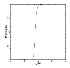
Figure 5. Calculated dependence of the residual polarization in an electron storage ring on the g-factor of the electron.<sup>25</sup>
