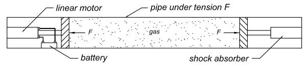
An important distinction between this and the previous example is that the pipe that confines the gas is now under tension F.
