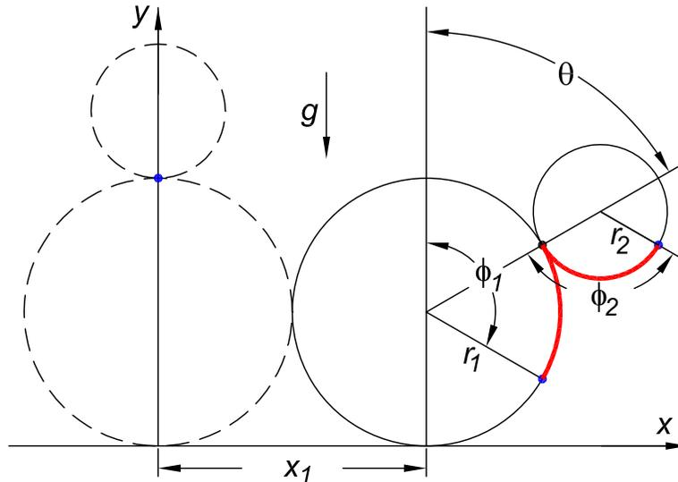
Meanwhile, if the upper cylinder, 2, rolls such that the line of centers (in the  $x$ - $y$  plane) makes angle  $\theta$  (positive clockwise) to the vertical, then the initial point of contact of the upper cylinder has rotated through angle  $\phi_2$ , measured counterclockwise from the line of centers, such that for rolling without slipping the arc lengths are equal between the initial
