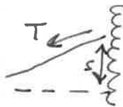
$$\sum F = 0 = -\underbrace{T s'}_{\text{STRING}} - \underbrace{K s}_{\text{SPRING}} \quad (\text{WATCH SIGNS!})$$
