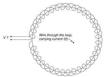
What is the voltage V(t) induced at the leads of the bent solenoid coil? Show that this voltage is independent of the exact shape of the coil, and independent of the position of the current-carrying wire. Give a physics reason why the return wire should pass down the center of the coil.
