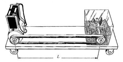
A battery drives a motor that in turn drives a paddlewheel via a belt drive. The paddlewheel turns in a water bath that heats up as a consequence. Hence, energy E is transferred from the battery to the water bath, and as a result the mass of the battery decreases by  $E/c^2$  while the mass of the water increases by the same amount, where c is the speed of light.<sup>2</sup>
