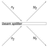
Hint: a relatively elementary argument can be given by recalling that the phase of a reflected photon (i.e., of the reflected wave from a single input beam) is  $90^{0}$  different from that of a transmitted photon [2]. Consider first the cases that one of  $n_{1}$  or  $n_{2}$  is zero.
