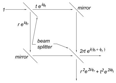
Then, the amplitude for transmission at the first beam splitter, followed by reflection at the second, is  $tr, e^{i(\phi_t + \phi_r)}$ , etc. Hence, the recombined beam that moves to the right has amplitude,
