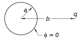
To apply this to the present problem, sketched in the figure below, note that the image wires of charge  $\pm q$  per unit length are both located to the left of the center of the inner conductor, say at distances  $r_a$  and  $r_b$ .
