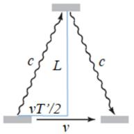
Here, the path of the light beam from the first mirror to the second and back has length cT' in the lab frame, while the first (bottom) mirror travels distance vT', Then,
