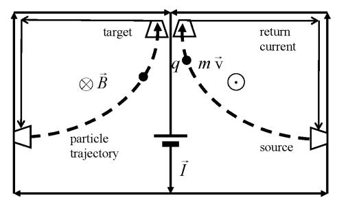
Positive ions are emitted "horizontally" and inwards from sources around a ring on the "vertical" wall of a conducting cylinder, and deflected upwards by the azimuthal magnetic field generated by a "downward" electrical current (driven by a "battery") in a wire along the axis of the cylinder. When the ions are collected at the (conducting) "top" plate of the cylinder, the latter experiences an impulsive "upward" force.
