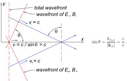
So, Slepian's form (1) is a valid electromagnetic wave, and in fact corresponds to the so-called  $TE_{10}$  mode of a rectangular waveguide, as discussed in sec. 2.1 below.
