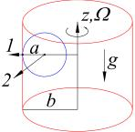
If  $\Omega = \dot{\phi}$  = angular velocity of the point of contact about the vertical,  $\hat{\mathbf{1}}$  points from the center of the sphere to the point of contact,  $\hat{\mathbf{z}}$  is vertical, and  $\hat{\mathbf{2}} = \hat{\mathbf{z}} \times \hat{\mathbf{1}}$ , show that the component equations of motion are,
