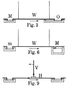
A horizontal wire W in Figs. 3 and 6, H in Fig. 9, was suspended from nonconducting strings, and it tips bent vertically downwards into cups of mercury, labeled M and O in Fig. 3. When a strong current flowed from right to left, via lead wires also dipped into the mercury cup, the central, horizontal wire was observed to move to the right.
