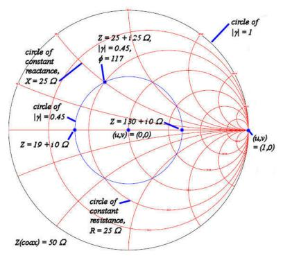
For ease of use, curve of constant resistance  $R_2$  and constant reactance  $X_2$  are also shown on the Smith chart, for a specified value of the (real) impedance  $Z_1$ . For this, we write,
