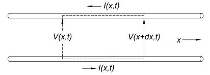
Next, the charge dQ that accumulates on length dx of the upper wire during time dt is (Cdx)dV in terms of the change of voltage dV between the wires and the capacitance C per unit length between the two wires. The charge can also can be written in terms of currents at the two ends of segment dx, so that,
