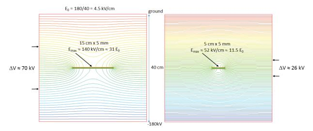
The figures indicate that the charging of the sharp corners of the insulator leads to closely spaced equipotentials there, such that the total potential difference between the "top" and "bottom" sides of the insulator is large ( $\Delta V \approx 70 \text{ kV}$  in the example on the left above, and  $\approx 26 \text{ kV}$  on the right).
