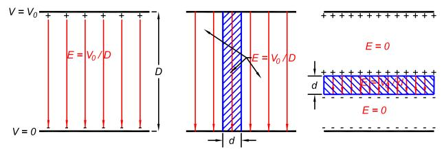
If the plane of the insulator is parallel to the field  $\mathbf{E}_0$ , and completely fills the gap of height D between the electrodes that establish that field, then the field inside the insulator is also  $\mathbf{E}_0$ , independent of the permittivities of the insulator or the medium surrounding it. See the middle figure above.
