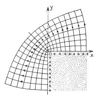
The electric field lines for this new problem are identical with the equipotentials (and *vice versa*) for the original problem of a conducting corner. From the figure above (p. 254 of [16]), we see that the potential (32) corresponds to an electric field that is parallel to the surface of the corner, as desired for the steady-state of a charged, rectangular insulator.
