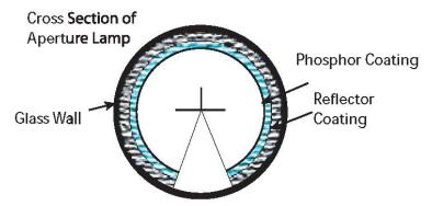
Phosphor molecules are excited by ultraviolet light emitted during the steady electrical discharge of the low-pressure gas inside the lamp, and subsequently de-excite via emission of visible light. Some of this light is absorbed and re-emitted by the phosphor. In this problem, assume that there are no losses in this absorption/re-emission.
