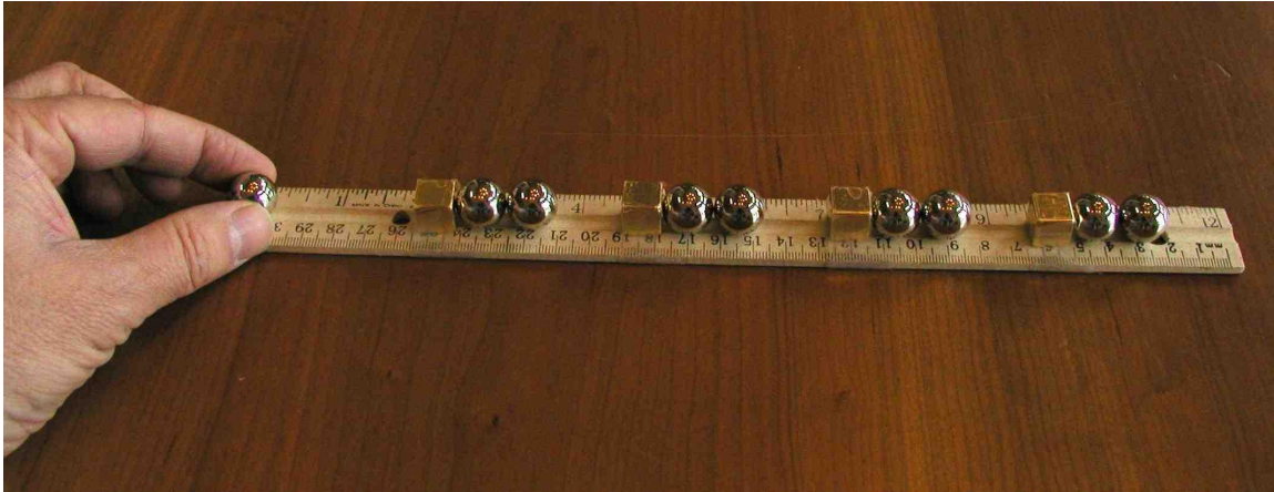
Figure 1: The magnetic linear accelerator, from Scitoys.com [1]
