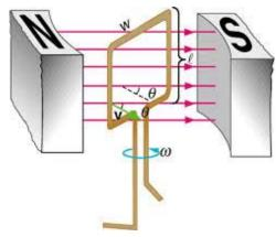
What is the electric field  $\mathbf{E}$  in the various segments of the rotating rectangle when angle  $\theta = 90^{\circ}$ , neglecting the small effect of the fields induced by the current that flows in this dynamo.
