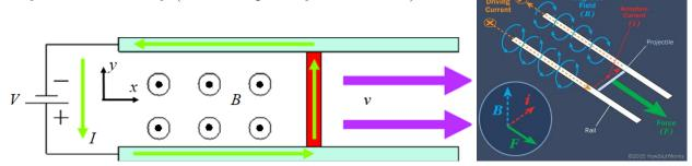
In these experiments with sliding contacts, the current density (for a given total current) at the sliding contact is not as large as that in experiments with a rolling contact, and the Lorentz-force explanation is largely satisfactory.<sup>14</sup>
