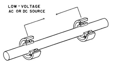
The motor can start from rest (although not all observers report this [1]-[24]), and rotates in either sense, if the current (AC or DC!) is large enough.
