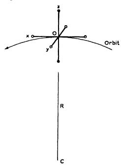
We use a rectangular coordinate system centered on the support point (O in the figure above, from [1]), with the z-axis along the vector  $\mathbf{R}$  from the center of the Earth to the
