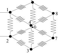
If the leads are connected to points 1 and 3, note that  $V_2 = V_4 = V/2 = V_6 = V_8$ . Thus, resistors 1-2 and 1-4 are in parallel and can be replaced by a single resistor of value *R*/2. Likewise, 2-3 and 3-4 merge into one with *R*/2, 5-6 and 5-8 merge into one with *R*/2, and 6-7 and 7-8 merge into one with *R*/2. Now it is "straightforward" to finish the analysis.
