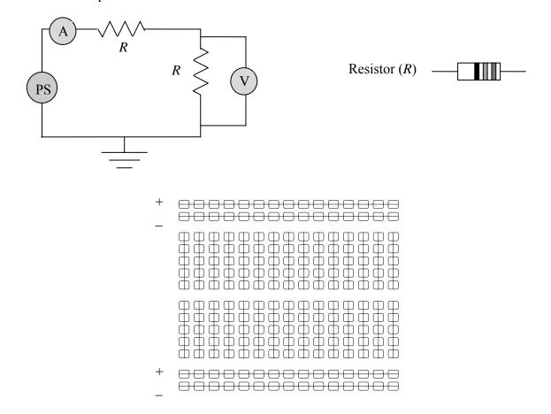
**2.** Given an ammeter, a voltmeter, a battery and an unknown resistor, draw the schematic of a circuit you would use to measure the resistance of the unknown resistor. What is the resistance, in terms of the measurements?
