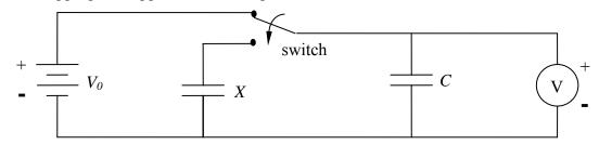
The voltmeter has a large but finite internal resistance. As a consequence the voltmeter discharges the capacitors slowly, which will cause an uncertainty in your determination of capacitance X if you wait too long to read the voltmeter. Deduce the value of the internal resistance of the voltmeter by observing the time dependence of the voltage across capacitors C and X.
