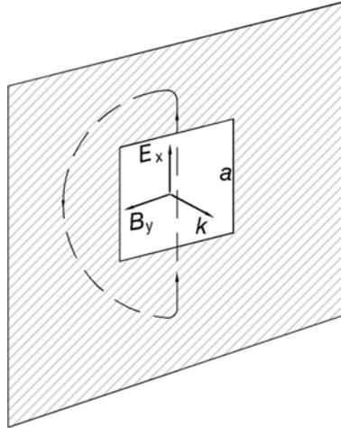
The electric field is essentially zero close to the screen on the side away from the source. Then, at time  $t = 0$ , the electric field in the aperture has strength  $E_x$ , so that integrating around the loop we have
