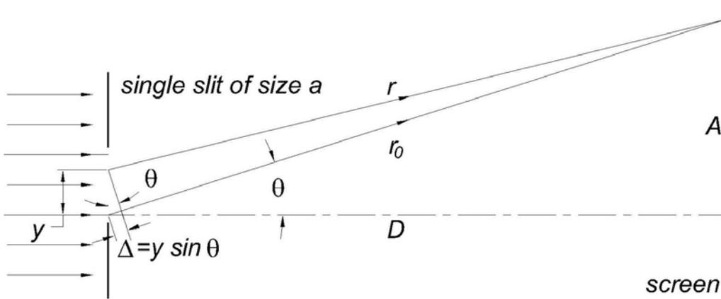
From the geometry of the similar triangles in the figure, we see that the length of ray  $r_0$  is related to that of ray  $r$  by  $r = r_0 - \Delta = r_0 - y \sin \theta$ . Using this, the combined field strength at the point on the screen is
