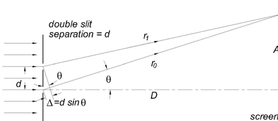
From the geometry of the similar triangles in the figure (and the assumption that  $A \gg d$  so that the rays are essentially parallel), we see that the length of ray 0 is longer than ray 1 by  $\Delta = d \sin \theta$ , so that  $r_1 = r_0 - \Delta = r_0 - d \sin \theta$ . Using this, the combined field strength at the point on the screen is
