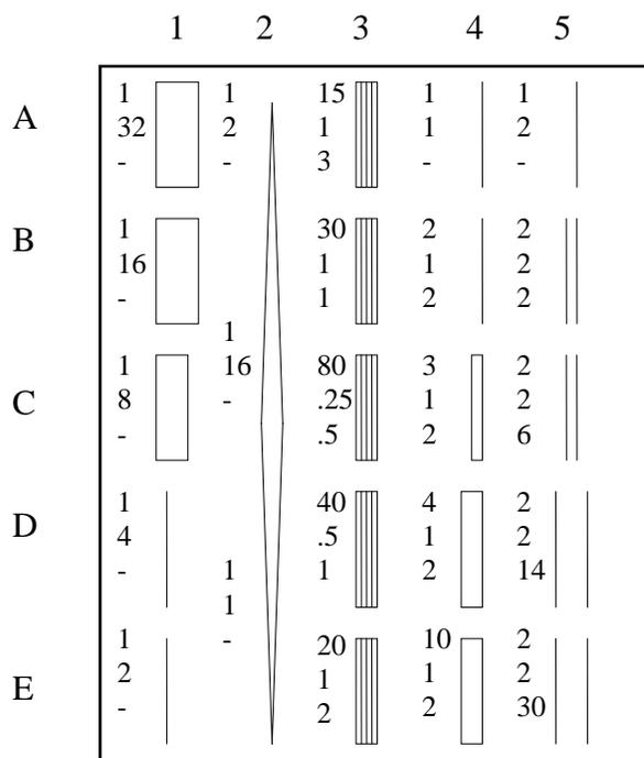
Complete your look at Young's double slit pattern by observing the patterns gotten by shining the laser onto the screen through a series of double slits, 5B, 5C, 5D, 5E, with increasing distance  $d$  between the slits. Sketch the interference patterns in your notebooks, and write down your qualitative observations.
