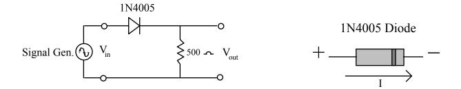
The rectified output voltage  $V_{\rm out}$ , is essentially all of the same sign, but is too bumpy to be very useful. As you can see on the oscilloscope, the diode has rectified the sinusoidal input voltage from the signal generator by "chopping off" the bottom half. This happens when the current will try to flow through the diode in the reverse bias and it is not permitted to flow that way by the diode.
