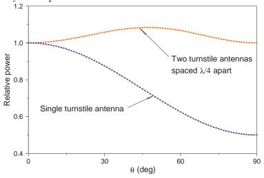
(b) But we can make the pattern even more isotropic by considering a vertical stack of turnstile antennas.
