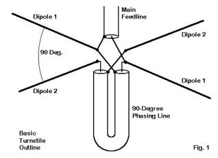
For simplicity, you may approximate the turnstile radiator as made of a pair of point dipoles of peak strength  $p_0$ , oscillating with angular frequency  $\omega$ , centered on the origin, one oriented along the x and the other along the y axis, with the second dipole driven 90° out of phase with respect to the first.
