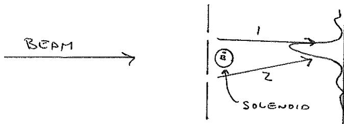
$$\text{For an ideal solenoid } \oint \vec{A} \cdot d\vec{l} = \int \vec{B} \cdot d\vec{s} \Rightarrow A_\phi = \frac{BR^2}{2\pi} \quad \text{for } r > R_{\text{Solenoid}}$$
