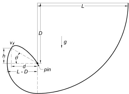
We seek the special case that the bob just passes over the pin, such that the string ends up wrapped 3/4 of the way around the pin when the bob finally comes to rest.
