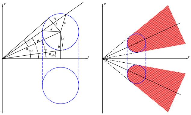
The vector potential of eq. (2) at  $(r, \theta, \phi)$  is nonzero along a ray from the origin for all  $r > r_1$  of eq. (4), *i.e.*, only within the "shadow", with,
