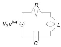
Deduce the Q of this circuit, and relate it to the electromagnetic field energy of the circuit.
