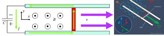
We take the capacitor C to be at x = 0 and the crosspiece (in red) at  $x = x_c \gg b$ , where the various wires of radius  $a \ll b$  lie in the plane z = 0, with x-segments centered on y = 0 and b. The magnetic field in the plane z = 0, between the x-segments and away from their ends, is approximately that associated with infinite-length wires,
